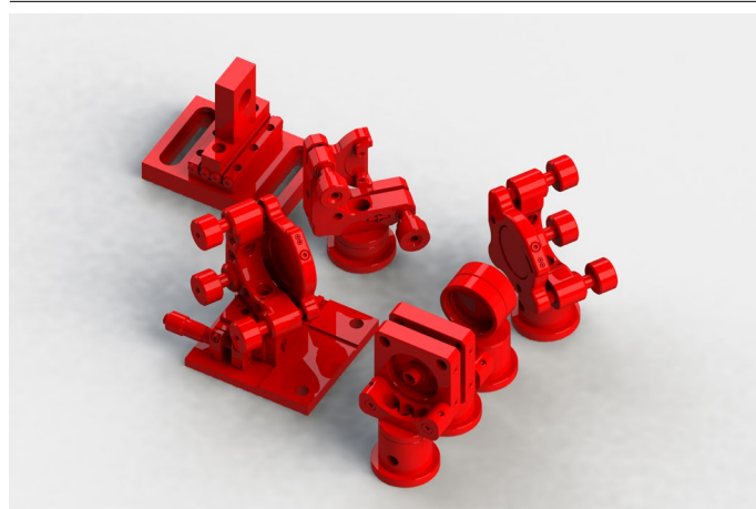
Fig. 7 | The fully assembled focus lock path. A fiber coupled NIR (808 nm) laser is connected to the fiber terminating adapter (bottom) and focused by a lens (occluded) onto the objective BFP via a pair of steering mirrors and cleanup/neutral density filters. The second steering mirror is on a manually adjustable translation stage to offset the beam at the BFP to achieve the condition for total internal reflection at the coverslip sample interface (for oil objectives) or to optimize for Fresnel reflections (for silicone oil objective lenses). The returned beam is picked off by a D-shaped mirror and captured on a quadrant photodiode (QPD). The QPD measures focal drift as a positional offset of the returned beam and sends a corrective signal to the objective lens piezo flexure stage accordingly. Mounting the QPD on a motorized stage allows refocusing during focus lock operation by translating the QPD.
